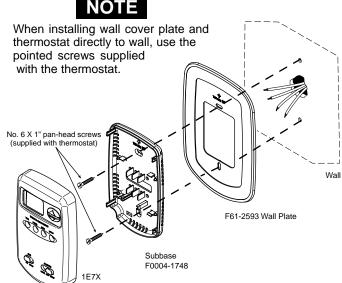
Figure 2. Mounting 1E7X vertical digital thermostat to wall.
